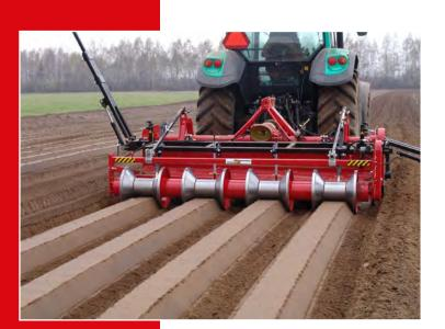
Built with a working width from 250 to 400 cm, required power from 140 to 240 HP and working depth from 15 to 30 cm. RSE-PLUS stone burier with bed former shaper is a professional machine used mainly by contractors and large horticultural companies that need to work in extreme conditions.
